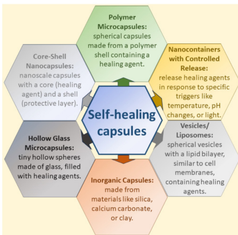
Figure 2: Types of self-healing capsules [4].
