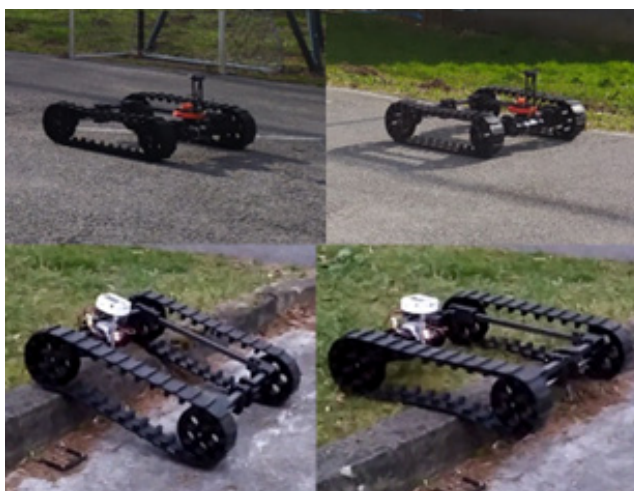
Figure 4: Tracked differential-drive UGV prototype tested for GPS navigation and remote control [13].
