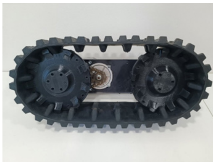
Figure 8: Assembled drive side showing integrated mechanical elements and DC motor.
