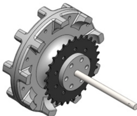
Figure 6: 3D model of the custom drive wheel assembly with integrated mechanical components.
