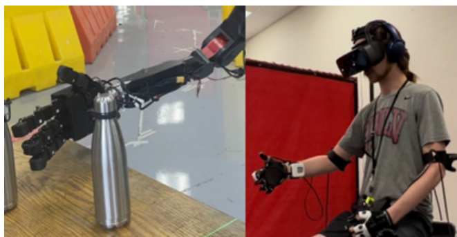
Figure 1: Human operator using Virtual Reality Headset and Haptic Data gloves (right) to control sensorized anthropomorphic robot hand (left).
