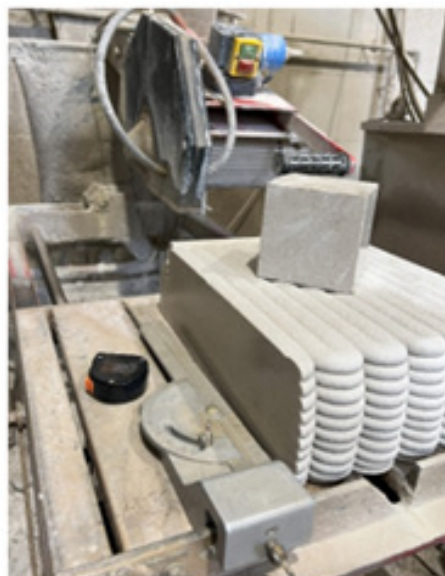
Figure 4: Cutting process of 100 mm cubes from the printed slab.
