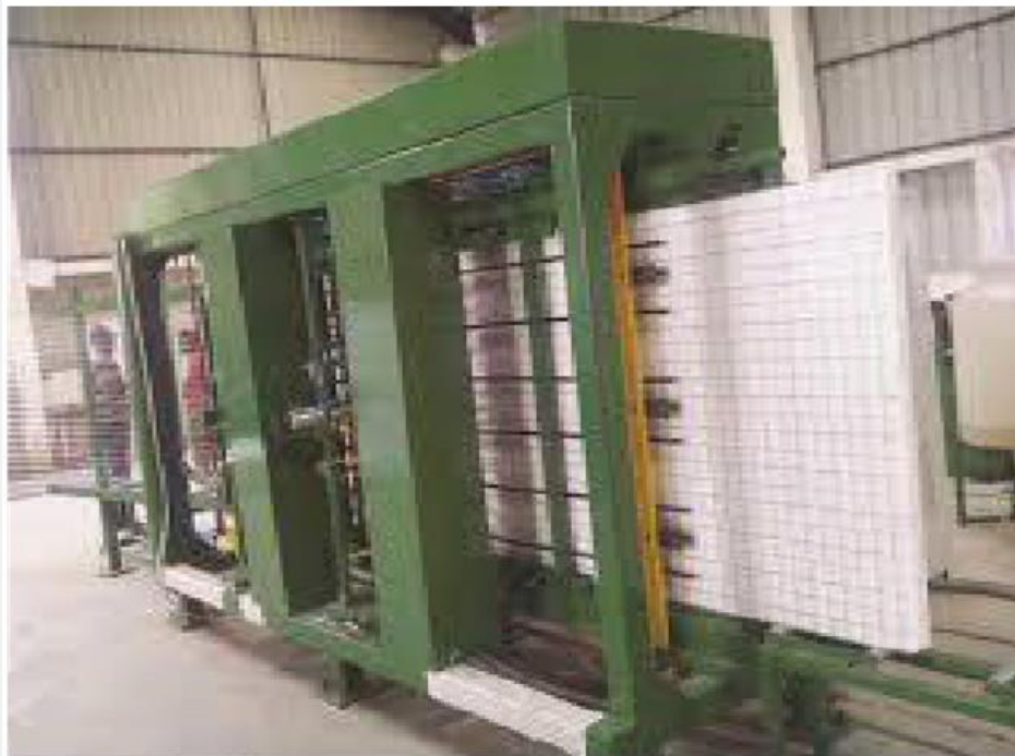
Figure 3: 3D-panel making machine.
