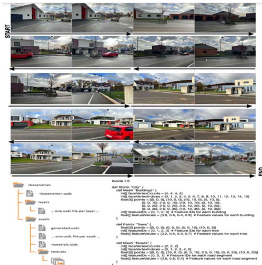
Figure 7: Dataset sample for VGE for 3D Geosimulation with the USD schema files.
