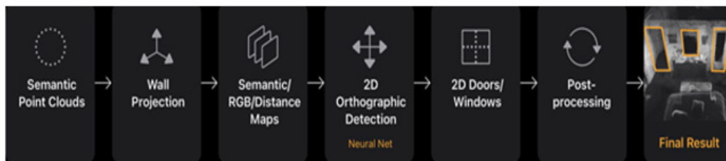
Figure 4: Doors and Windows Detection Processing.
