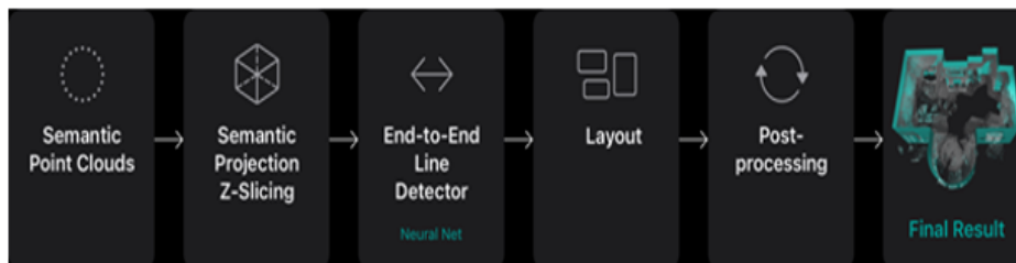
Figure 3: Walls and Openings Detection Processing.
