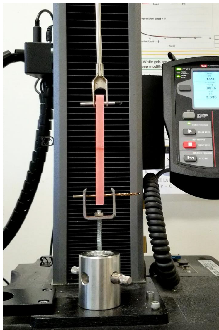
Figure 5: Tensile strength test setup with the specimen (P-PMMA) in vertical position.
