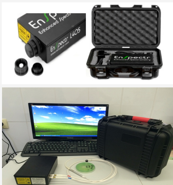
Figure 2: Modifications of The InSpectr M-Device with Optical Fiber and Nozzles for Working with Biological Fluids, Smears and Biopsy Material.
