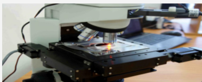
Figure 1: Raman Microscope "InSpectr M532" and 2D Scanning Motorized Movement.
