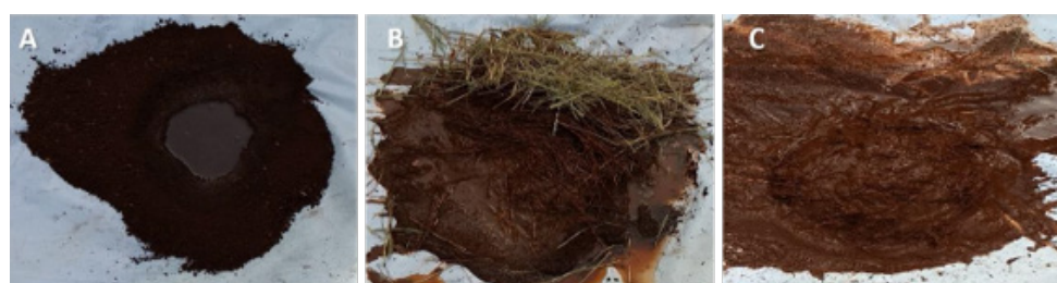
Figure 6: Preparation of the mixture for the adobes: A) soil and water, B) fiber incorporation and C) adobe mud.
