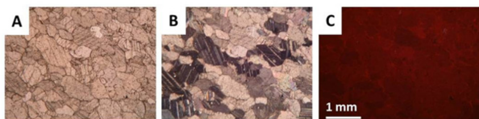
Figure 13: Representative photomicrographs of the marble. A) in plane polarised light. B) in crossed polarised light. C) CL-pattern.
