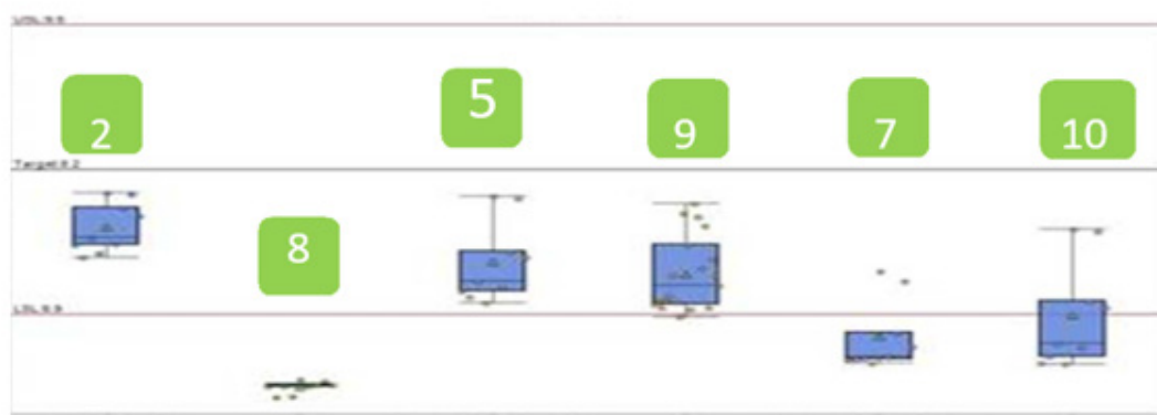
Figure 3: correlation between electrical parameter ( \text{mV}/\text{cm}^2 ) and SiC over etch. Sample 2: ME + OE with CO; Sample 8: ME + 20% OE; Samples 5,9: ME + OE 10%; Samples 7,10: POR.
