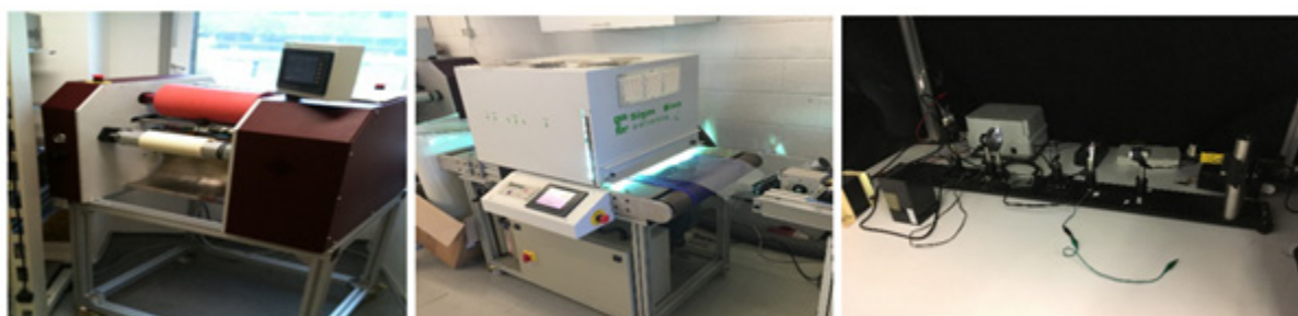
Figure 1: PDLC film coater/laminator(left), UV-IR curing conveyor (centre) and electro-optical system (right).
