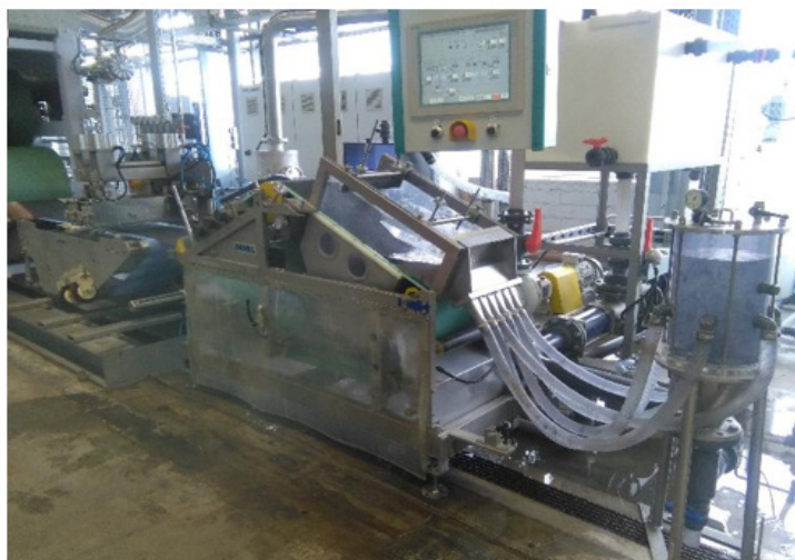
Figure 1: Pilot plant for CF nonwovens from Andritz Küsters GmbH (Krefeld).
