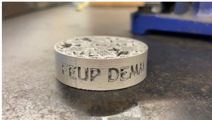
Figure 1: Gear bearing optimized for weight reduction, by using lattice structures.
