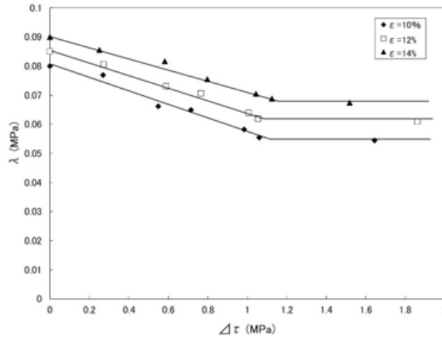
**Figure 3:** Stress decrement ( $\Delta\tau$ ) vs.  $\lambda$  for non-irradiated NaBr single crystal at 193 K.
