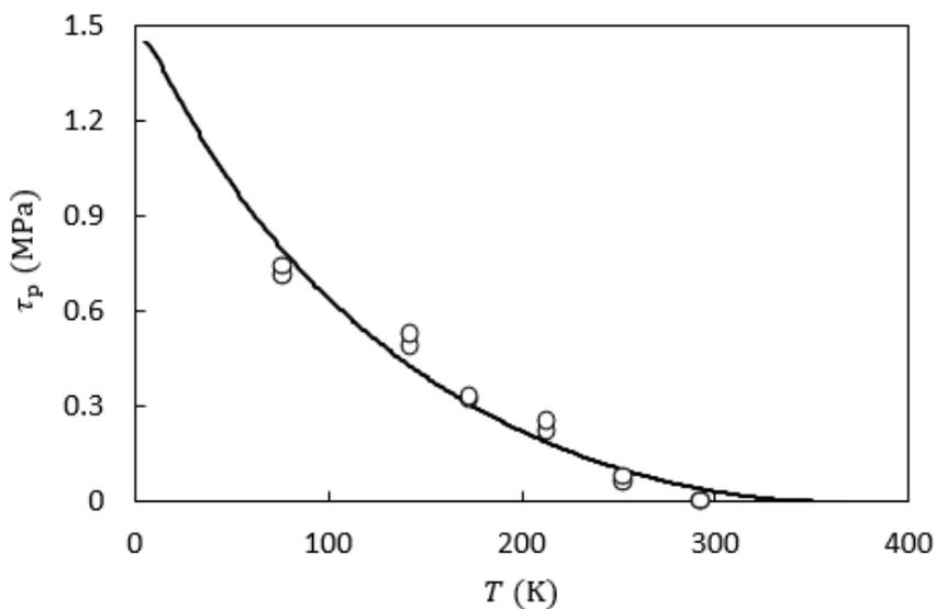
Figure 5: Dependence of  $\tau_p$  on temperature for X-ray-irradiated NaBr single crystal. The solid curve is given by numerical calculation [14].
