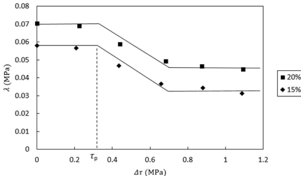
**Figure 4 (a):** Stress decrement ( $\Delta\tau$ ) vs.  $\lambda$  for X-ray-irradiated NaBr single crystal at 173 K.
