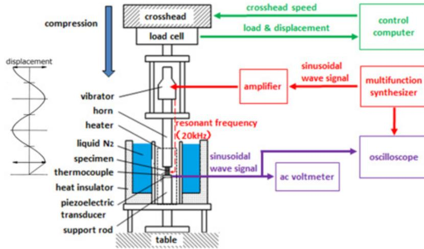
Figure 1: Experimental apparatus: schematic block diagram of apparatus system.
