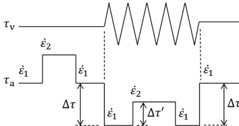
Figure 2: Variation of applied shear stress,  $\tau_a$ , when the strain-rate cycling between the strain rates,  $\dot{\epsilon}_1$  ( $1.1 \times 10^{-5} \text{ s}^{-1}$ ) and  $\dot{\epsilon}_2$  ( $5.5 \times 10^{-5} \text{ s}^{-1}$ ) are carried out under superposition of ultrasonic oscillatory shear stress,  $\tau_v$ .
