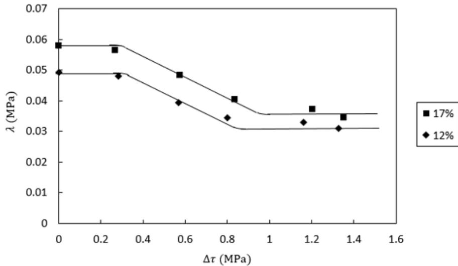
Figure 4 (b): Stress decrement ( $\Delta\tau$ ) vs.  $\lambda$  for X-ray-irradiated NaBr single crystal at 213 K.
