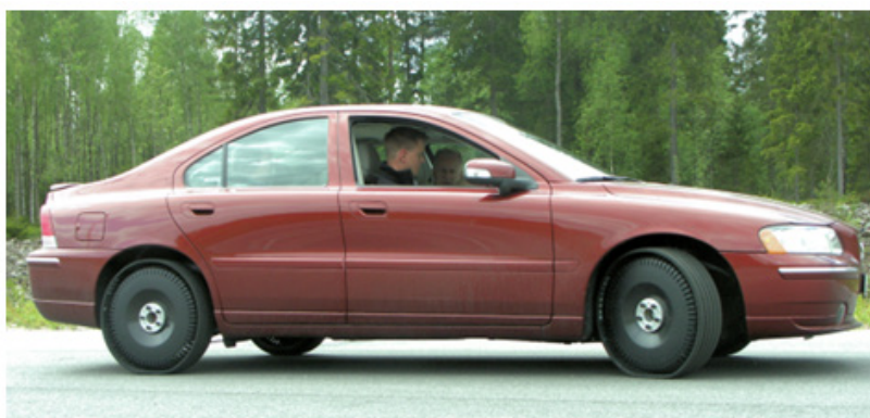
Figure 3: The Composite Wheels mounted on a Volvo car for various tests. Photo by the author.
