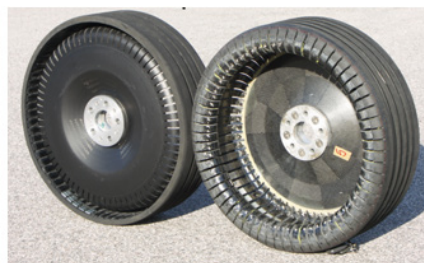
Figure 2: The airless tire (Composite Wheel) final prototypes produced in the author’s project. The left tire shows the outside of the tire; the right tire shows the inside (to be mounted towards the car chassis). Photo by the author.
