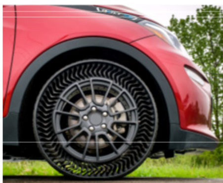
Figure 4: The Uptis airless tire mounted on a Bolt electric car by GM, presented by Michelin in 2019. Photo by Michelin, used with permission.
