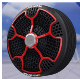
Figure 6: Hankook's iFlex airless tire concept. Photo by Hankook, used with permission.
