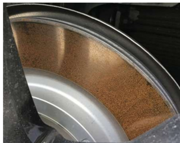
Figure 3: Corroded friction surface of an electric vehicle's brake disc.
