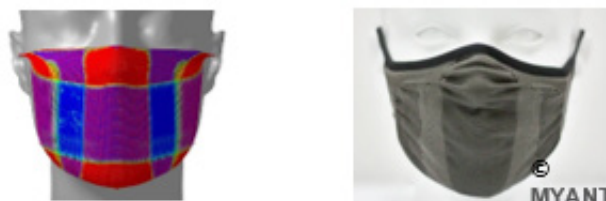
Figure 9: Draping of a face, given in STL format or as a point cloud, using a stretchable membrane and stiffening it with double yarns or dense patterns to achieve the required shapes and functionality, demonstrated on the example of a knitted mask.
