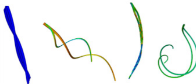
Figure 2: Simulation of the anisotropic pre-strain in yarns (one is pre-stained, another not) with different boundary fixations.
