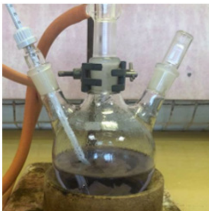
Figure 7: DMSO dye removal showed the greyish-purple solution and the discolored wool at the bottom of the flask.
