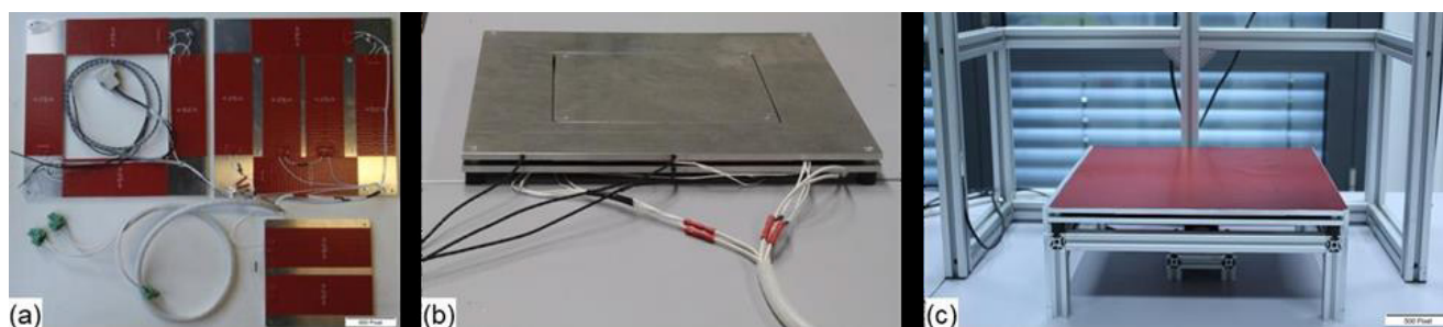
Figure 1: Calorimeter plate, framing and base plate: heating mat configuration (a), mounted. with black cables for temperature sensors and white cables for heating mats (b), experimental setup in the laboratory (c).
