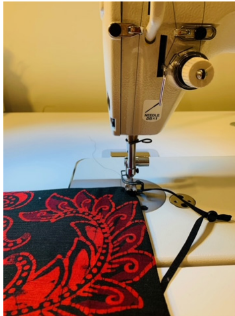
Figure 3: Mask making process: Sewing the fashion fabric and the earpieces to lining of the mask. The nose bridge has been sandwiched between the lining and the fashion fabric at the top of the mask (not shown in the photo).
