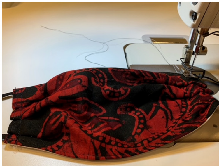
Figure 4: Mask Making Process: Stitching the pleats on each side of the mask.
