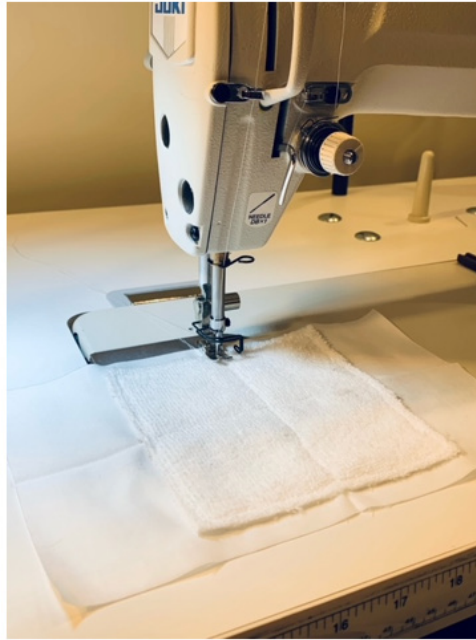
Figure 2: Mask making process: Attaching the electrostatic filter to the lining of the mask.
