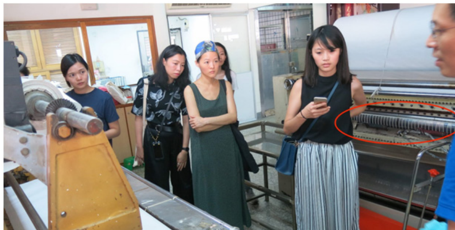
Figure 7: Factory visit at Sinta, New Taipei City, 2016. The clamps in red circle control the density of the pleats.
