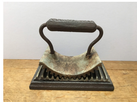
Figure 6: Hand pleating machine: rocker model. Geneva Hand Fluter (1868) cast iron, 9cm×15cm× 14cm.
