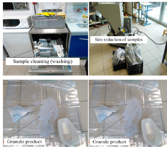
Figure 4: Cleaning, size reduction process of styrene based polymeric materials respectively.
