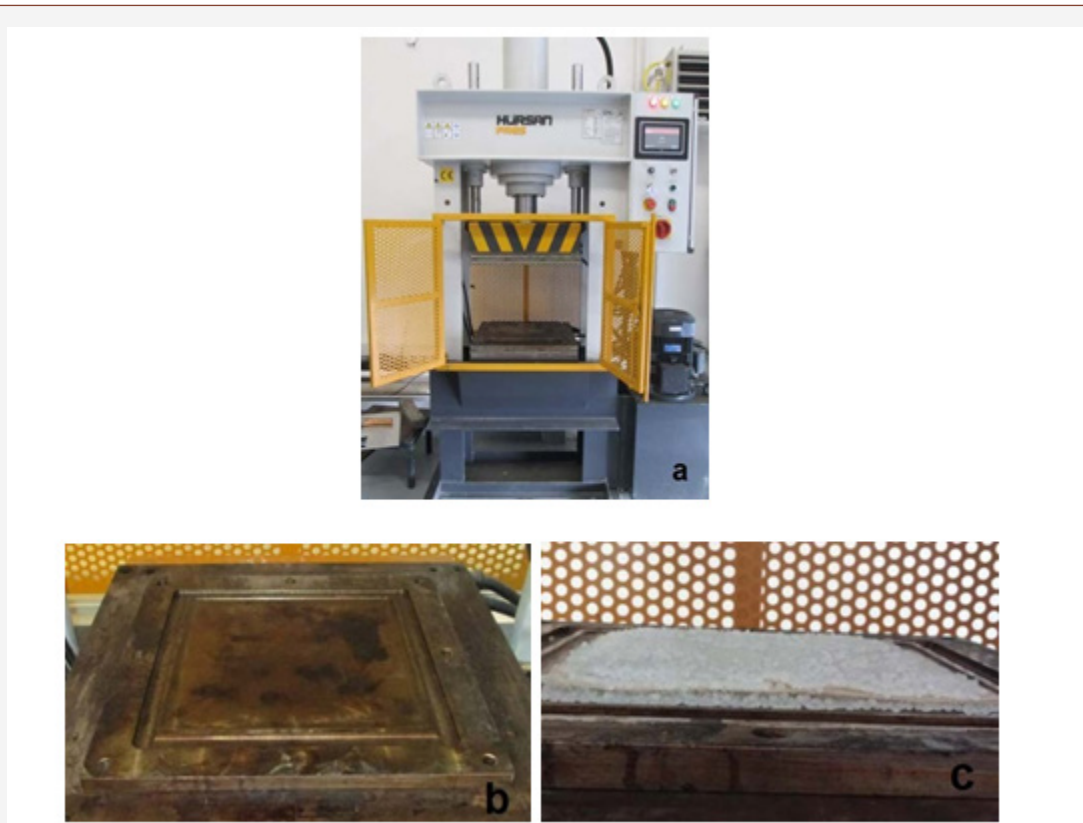
Figure 1: Used in composite material production (a) hot press machine (b) lower mold (c) Stacking of the polymer chips (PP-PE) and sisal fibre.
