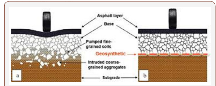
Figure 17: Soil Separation by geosynthetics.
