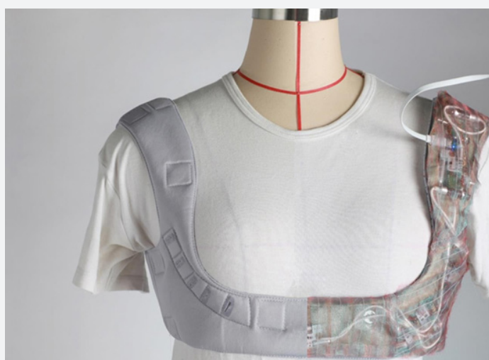
Figure 4: The finished second prototype designed to go under the breast area. The inside of the device is exposed on the right and covered on the left.
