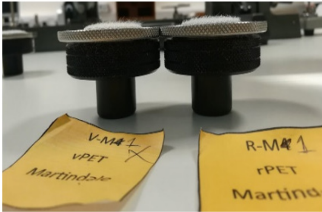
Figure 7: Side view of the V-PET and R-PET fabrics after abrasion resistance test.
