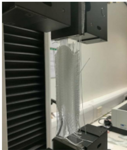
Figure 3: Experimental test setup of dynamic yarn strength test.
