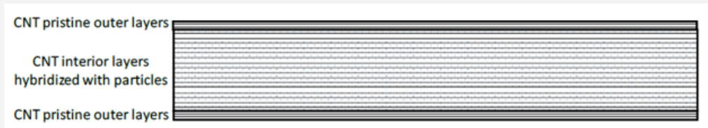
Figure 8: CNHT functional textile. The CNT sheet side view illustrates many layers from hundreds of revolutions wrapping CNT sock onto a drum at 20 RPM for 2-3 hours. The CNT hybrid sheet can be functionally graded with different concentrations of particles for controlling porosity and tunable properties through the thickness of the sheet. Also, the top and bottom layers are pristine to reduce the release of particles from the interior of the sheet.
