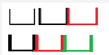
Figure 6: Continuous unit cell with the same length of single U type and different U type number.
