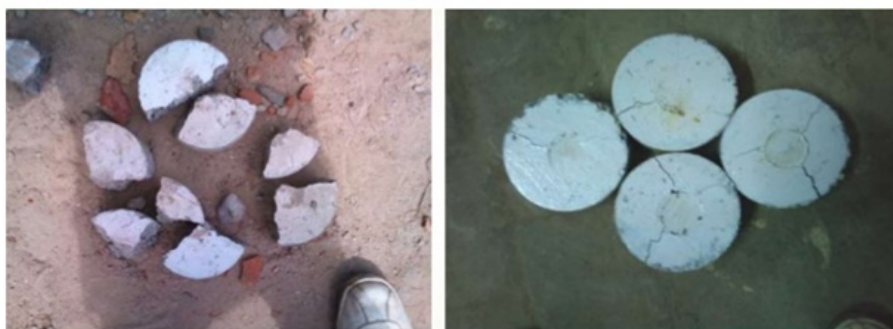
Figure 3: Mechanism of failure of cylinders under impact testing.
