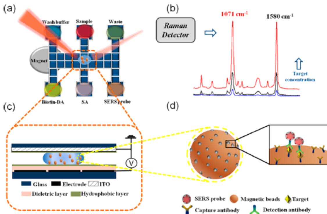
**Figure 6:** Schematic representation of the DMF-SERS assay (a) DMF-SERS method and bottom plate of DMF chip. (b) SERS peaks for the Raman tag. (c) Side view of the DMF chip coating a droplet of magnetic beads. (d) The sandwich biosensing approach [73].
