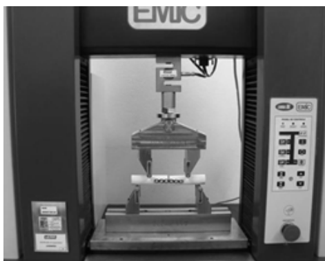
Figure 5: Device used to carry out the tests, showing the moment of assembly with four support points.
