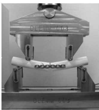
Figure 6: Moment of assembly failure during the static four-point flexion test.
