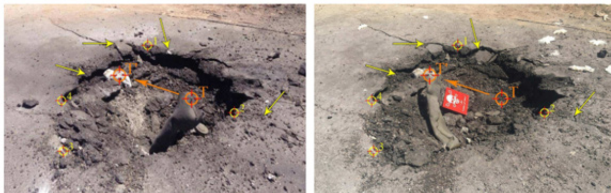
Figure 1.1: Comparison of the images (A_4) (left panel) and (B_2) (right panel). The observed differences in the crater shape are marked by yellow arrows. The orange arrow shows the bending direction of the pipe in image (B_2) . To make the comparison easier, we have made small perspective distortions of the image (A_4) (by approximately 10%) in order to make locations of four points (1–4) on the border of the crater exactly match in two images.
