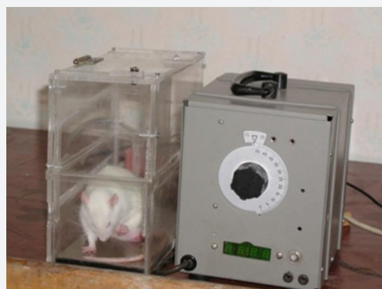
Figure 1: The “hot plate” setup for determination of pain threshold of rats.
