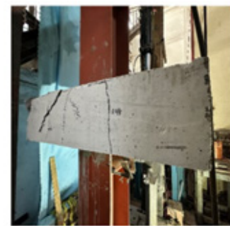
(c) Damage to the anchor end beam
