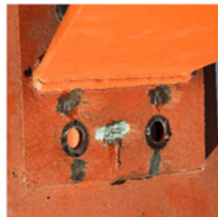
(b) Cracks appear in the weld seam
