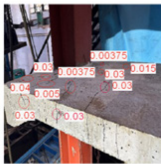
(b) Damage to the top surface of the floor slab
