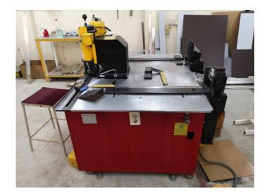
Figure 1: Bus bar bending machine.
