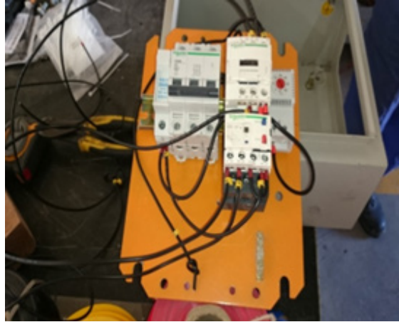
Figure 11: Wiring of the prototype according to line diagram.
