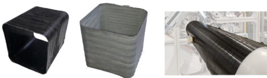
Figure 13: Structural parts from feasibility studies (left square profile, right cylindrical component).
