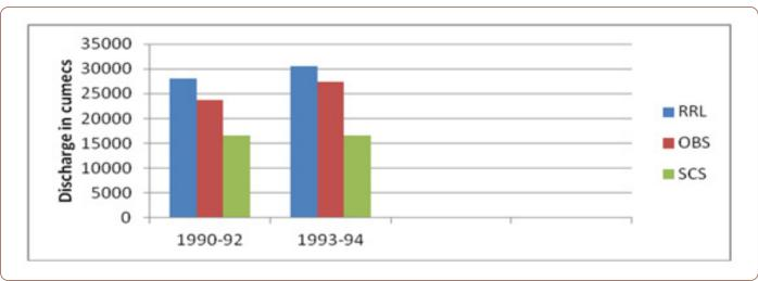
The SCS CN model gave the NSE during 1990-92 as 0.673 and 0.752 for the years 1993-94. The coefficient of determination values was 0.742 and 0.764 for the respective periods. The AWBM RRL model gave the NSE during 1990-92 as 0.852 and 0.890 for the years 1993-94. Clearly it can be seen that the AWBM RRL model slightly over predicts the discharge and the SCS CN under-predicts. The AWBM also shows good match between the simulated and observed discharge.
