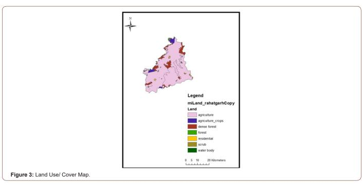
Using the attributes of the soil map and the land use/cover maps, the maps were merged and layered together so as to derive the composite curve number. The CCN was found out to be 77 for the bina basin.
