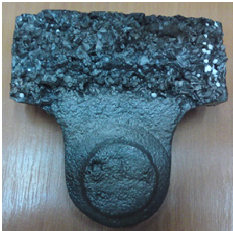
Figure 2: Hammer with as-cast non-oriented carbides.
