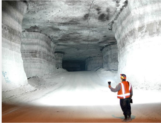
Figure 1: Stable pillars in a limestone mine at a depth of cover of 275m (900 ft). Slightly concave pillar ribs formed as a result of minor spalling of the hard, brittle rock.
