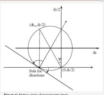
Figure 1: Mohr's circle of incremental strain.
