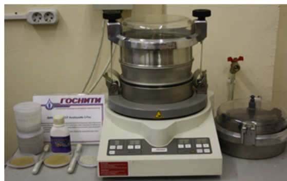
Figure 1: Fractionation of powders in a vibrating screen «Analysette 3 Pro»; the powder left is the original; in the center – processed, it became lighter; right powder companies «IKSAR»; in vials tribo-active «Sarnowski» and «RVD»; in jars powders CFG from Georgia.
