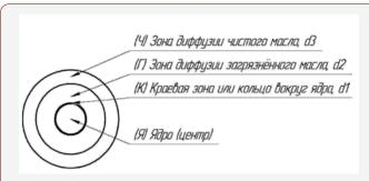
Figure 1: The composition of the oil spots on the filter paper laboratory].
