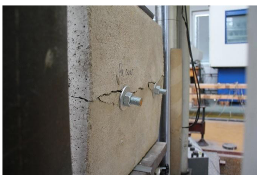
Figure 4c: Significant deformation of the textured layer and bending of the steel pins transferring the loads is visible.
