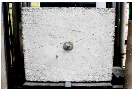
Figure 4d: All cracks in the element passed through the location of the connector, i.e., through the area of stress concentration and changes in their trajectory. The crack has been graphically redrawn.
