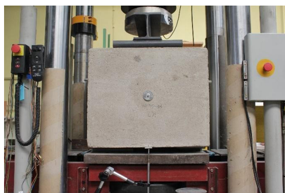
Figure 4a: Prior to the commencement of testing and continuously during the test, the symmetry and alignment of the pair of moulds were verified using a laser measurement system. The verification was carried out both in the plane parallel to the facing layer and in the plane perpendicular to it (i.e. in the transverse section of the moulds). Displacements were measured using displacement sensors installed beneath a steel plate fixed to the underside of both facing layers ("front" and "rear" with respect to the observer).
