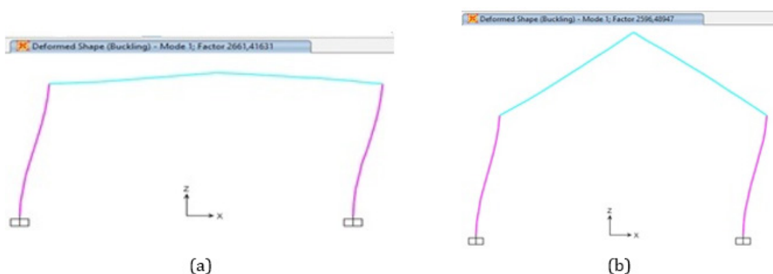
Figure 7: Critical buckling load of steel frame with rafter slope a) 5o, b) 35o
