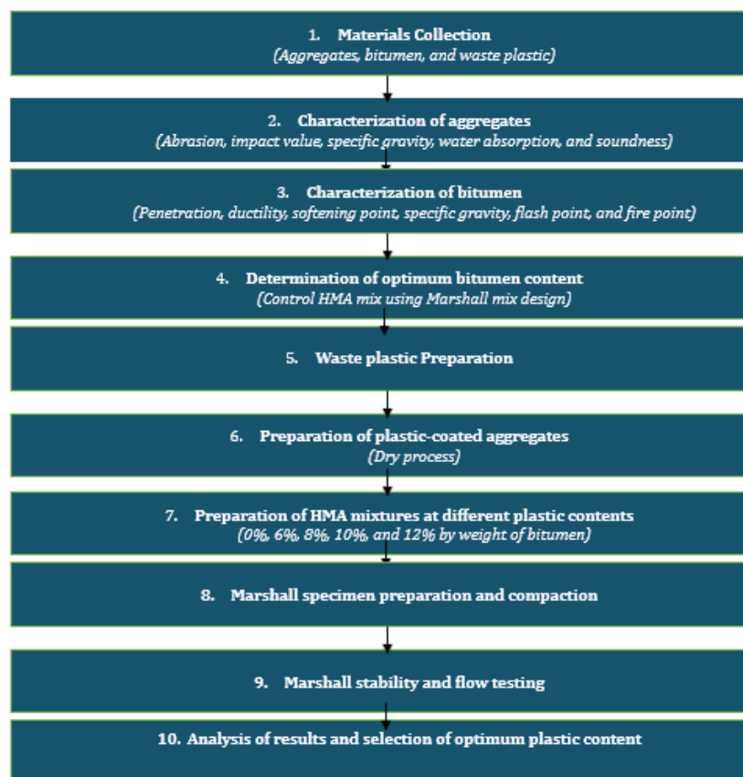
Figure 1: Experimental workflow for preparation and evaluation of waste plastic-modified hot mix asphalt.
