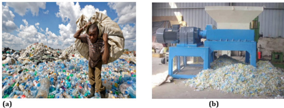
Figure 3: Waste plastic preparation: (a) collected waste plastic, (b) cutting/shredding process and shredded plastic particles.
