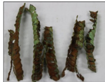
Figure 5: Condition of epoxy coating in a demolished bridge deck after about 25 years of service.
