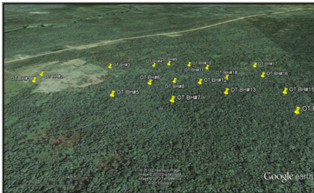
Figure 1: Orthogonal view of the Satellite Imagery of Federal University Site, Otuoke Bayelsa State, showing the distribution of the Boring points.
