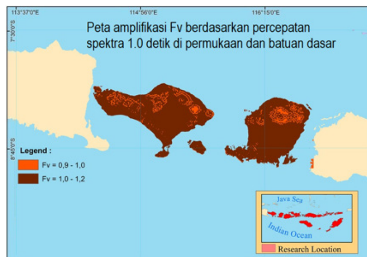
Figure 9: The Fv map, calculated based on spectral acceleration map data on the ground surface divided with spectral acceleration map data in the base rock for 1.0s period.
